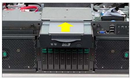
Figure 22: Inserting the tape drive
